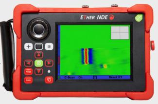
Area of Inspection: Fuselage Probe: Surface & Sub-Surface
