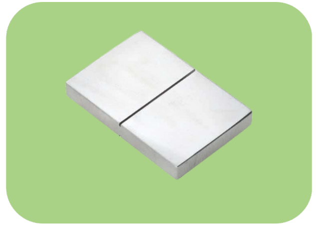
Aluminium sensitive test block
