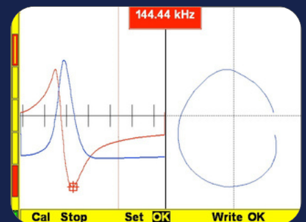
Air calibration for Resonance mode probes.
